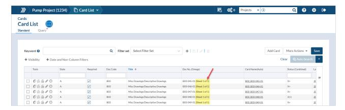
Sheet Adder is included in the internal document number but it can be removed from the Project Configuration page (Project Menu > Set Up > Project Configuration). Under the "Main" tab, expand the "Other Settings" section and set the "Display sheet adder for manual cards" value to **No.**
